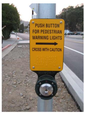
Activated pedestrian signals require pedestrians to push a button for signal recall
